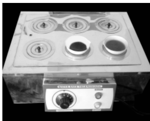
Plate 3 : Water bath used for aqueous extract preparation
