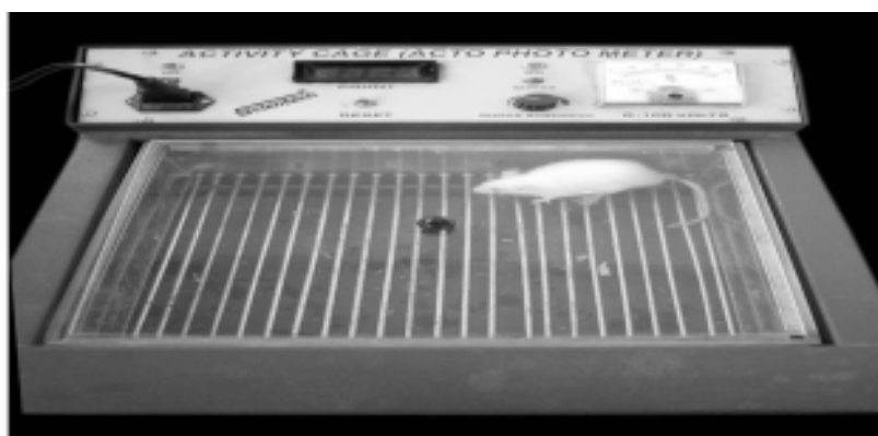
Plate 6 : Actophotometer - Used for Study of Motor inco-ordination
