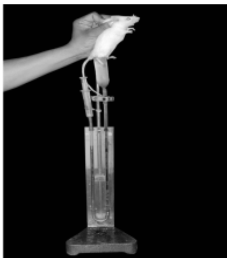
Plate 7 : Fabricated Plethysmometer used for acute inflammation measurement
